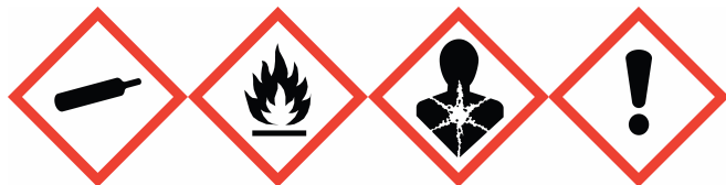
Compressed Gas Flammable Health Hazard Irritant
