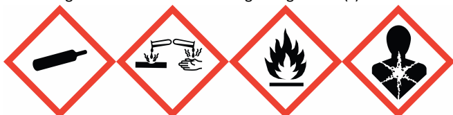
Compressed Gas Corrosion Flammable Health Hazard
